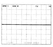
WFM ERROR is issued because 10 WFM is not a valid waveform memory address with the present conditions.
