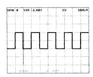
Point 102 is set at the designated vertical level. (If necessary, adjust the STORED INTensity.)
